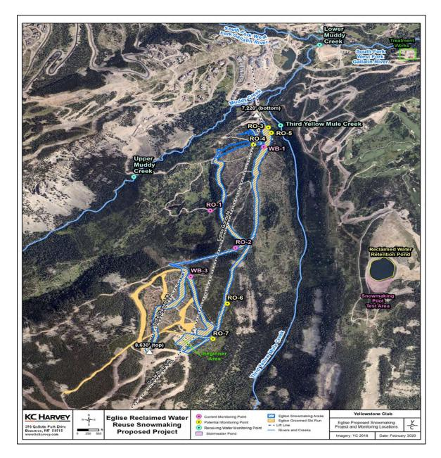
The existing 84 million gallon (MG) reclaimed water retention pond is located to the east of Eglise Mountain and holds reclaimed water from the BSCWSD and the YC treatment works. Reclaimed water from the BSCWSD is pumped uphill via a 7.5-mile-long force main to the YC retention pond to consume approximately 75% to 80% of the pond water volume.
